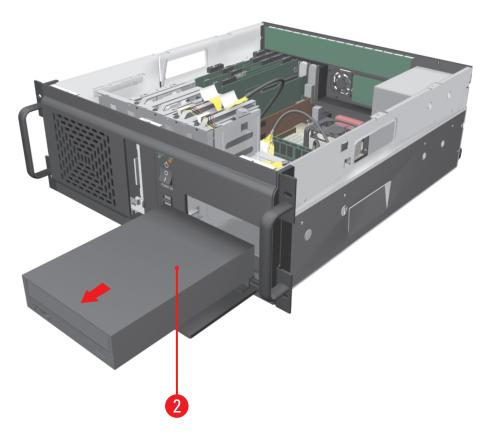
Figure 10. Removing the Existing Optical Drive
